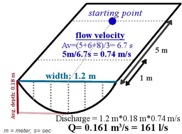
Figure 2 – The cross-section area and the float
